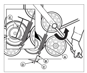
Figure 51. Mower Belt Idler Spring Length
